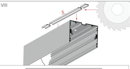
Attach the cover (5) between the holes for the fasteners leaving 5 mm space between the cover sections.
