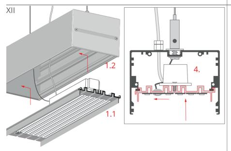
Connect the power supply (4) to the power cable.
