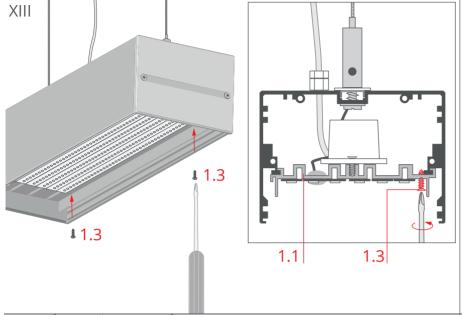
Secure the extrusion item (1.1) against slipping out by screwing the locking bolts (1.3) into the pre-drilled holes.
