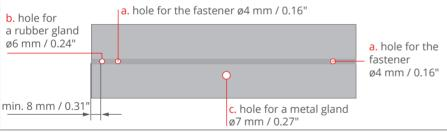
a. On both sides, from the side of the profile cross-section, thread the sockets for end cap bolts to a depth of approx.
