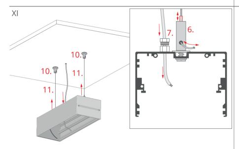
Fasten the extrusion on steel wires (11) to the ceiling fasteners (10). The suspension length can be adjusted by pressing the upper part in the fastener body (6).
