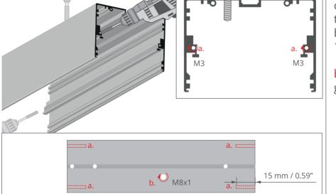
b. Thread the hole for the metal gland (M8x1 tap).
